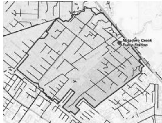
Tributary area of Matadero Creek Storm Water Pump Station (storm runoff from the outlined area is discharged to Matadero Creek via the dark storm drain pipelines that connect to the pump station).
