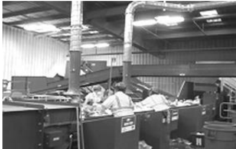
Workers ease the separation of items here on the line, with vacuum tubes above taking plastic bags.
